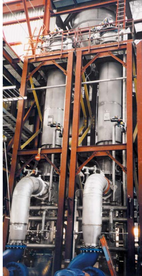
*Vertically installed, multi-pass membrane modules in a multi-stage system design. Vertical configuration conserves floor space.*
