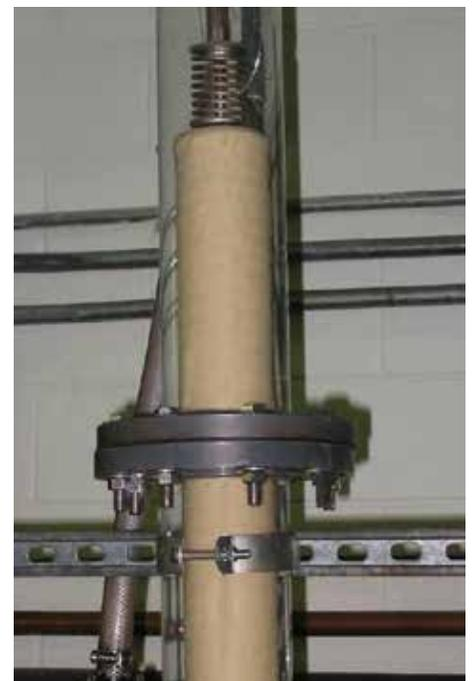
Top photo: Environmentally conscious Graver properly handles all waste from powdered resin processing. Bottom photo: Septum showing evenly distributed, uniform precoat layer across entire length.
