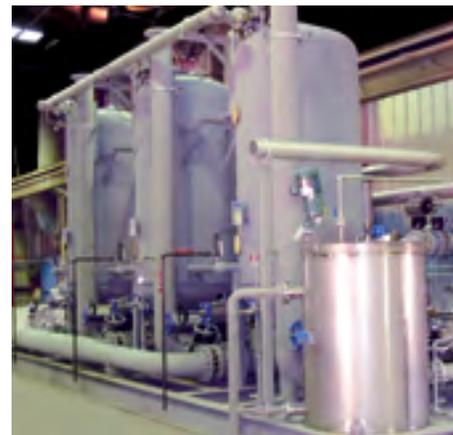
*Preferred over standalone filtration or deep bed ion exchange systems, state-of-the-art Powdex precoat filter demineralizers suit new or retrofit installations.*
