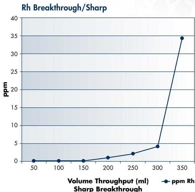
Rapid adsorption kinetics, lower flow rate unlikely to improve capacity.
