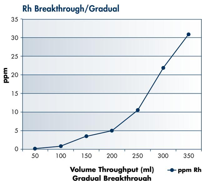
Limited Kinetics, a lower flow rate may help improve capacity. **Tip:** In general, conditions affecting the solubility of the compound and contaminant, such as time, temperature, and solvent type, will also influence adsorption kinetics, loading capacity and selectivity.
