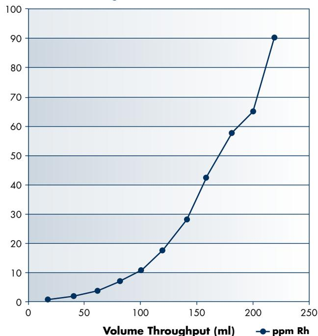
**INTERPRETATION/SCALE-UP PROJECTION:** From the breakthrough curve, the estimated volume of composite sample with a Rh level of  $\leq$  40 ppm is ~220 ml. The amount of purified API in 220 ml is 5.5 grams. Using linear mass based scale-up projection, the amount of API that can be processed to a satisfactory purity level with the various size cartridges is shown below. The gradual breakthrough suggests that reduced flow rate may help increase capacity.
