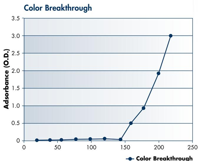
**INTERPRETATION/SCALE-UP PROJECTION:** From the breakthrough curve, the estimated volume of composite sample with a color of  $\leq 0.15$  adsorbance unit is  $\sim 240$  ml. The amount of purified API in 240 ml is 6 grams. Using linear mass based scale-up projection, the amount of API that can be processed to a satisfactory purity level with the various size cartridges is shown below. The sharp breakthrough suggests that reduced flow rate will not markedly increase capacity.
